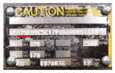
Next, we need to determine the seal type. The position (18th) and type of seal designation are shown below.
