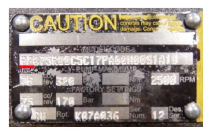
The design of the pump determines if the we support the seal kit. The design/series is in the bottom left hand side of the pump tag. This number is marked with a red line. If that part of the pump is damaged, the serial number (green line) can be used to determine the pump design. 60, 75, 105 size pumps with 11 design or higher are current pumps, and 145 size pumps with 12 design or higher are current too. All others are obsolete, and need to have the whole pump replaced.
