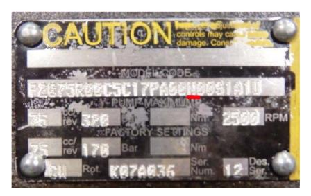
PLEASE NOTE: Before we select our seal material, it is a good practice to determine if the pump as after 12/1/2013, or ask the customer if the system fluid is compatible with Viton shaft seal material. Refer to PC00049 for the details. After 12/1/2013, all pumps were built with viton shaft seals. The coding for a complete Buna seal kit is letter B for a single shaft seal and Q for a double shaft seal.
