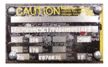
The pump displacement (75), the seal type (N), Design 12, and the port type (A) have been identified. There is enough information to select the seal kit. Below is the spread sheet with the old seal kits and new part numbers.
