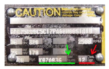
Next, we need to determine the displacement of the pump. The model code choices are below:
